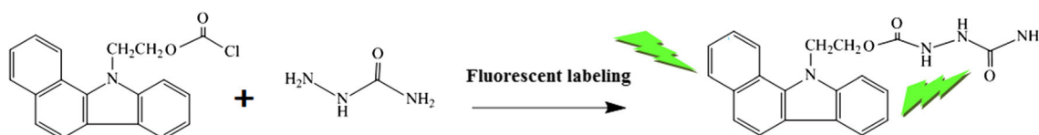
Fig. 2 The fluorescent labeling scheme for BCEC with semicarbazide (SEM) under the optimum conditions
