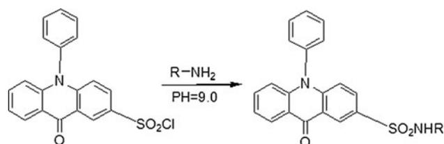
**Fig. 2** Derivatization scheme of PASC with aliphatic amines
