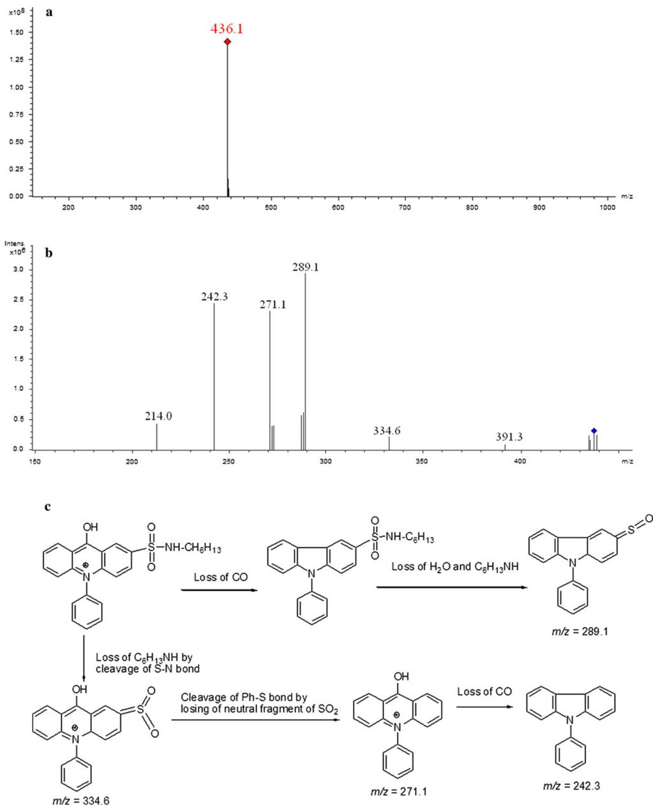
**Fig. 6** **a** MS, **b** MS/MS and **c** cleavage mode for representative PASC-hexylamine derivative
