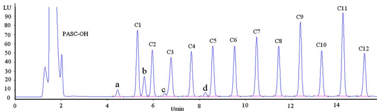
**Fig. 5** Chromatogram for the separation of standard aliphatic amines derivatized with PASC. Column temperature is set at 30 °C; flow rate = 1.0 mL min<sup>-1</sup> C1 methylamine, C2 ethylamine, C3 propylamine, C4 butylamine, C5 pentylamine, C6 hexylamine,
