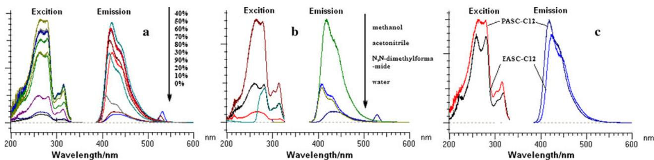
**Fig. 3** Fluorescence intensity of PASC-C12 derivative in the presence of varying amount of acetonitrile (a); the effects of solvent on the fluorescence intensity of the PASC-C12 derivative (b); fluorescence spectra of PASC-C12 ( $\lambda_{ex}/\lambda_{em} = 265/418$  nm, PASC-C12
